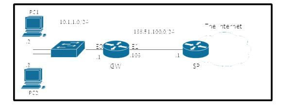
NAT has been configured on the router 'GW' and the IP addresses of router 'GW' have been configured properly. Users of PC1 and PC2 are able to ping the IP address 198.51.100.1 but are unable to reach any other IP addresses on the Internet. The ISP confirmed that their configuration is correct. Which option would likely correct the problem?
