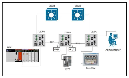
CIP Implicit messages from I/O#1 are being marked IP DSCP 47 by the endpoint and this marking is trusted by L2SW4. L2SW4 is configured to map DSCP 47 to output queue 1 threshold 1. You have received feedback that some of these messages are not being received. Executing the show mls interface GigabitEthernet statistics command on L2SW4 results in:
