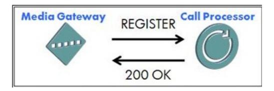
The figure shows part of a SIP transaction between a media gateway and a VCX Call Processor service. Which SIP role does the VCX Call Processor service play in the transaction?
