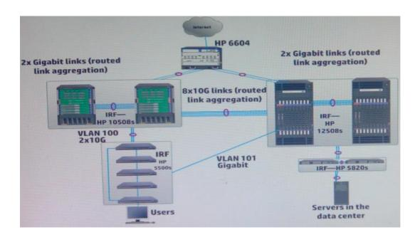
The exhibit shows the topology for an enterprise LAN with an on-site data center. The intelligent Resilient Framework (IRF) group of HP 5500 Series switches supports a group of computers that require very high availability to the data center. Therefore, the customer has requested a backup gigabit fiber link implement Open Shortest Path First (OSPF) in a single area.
