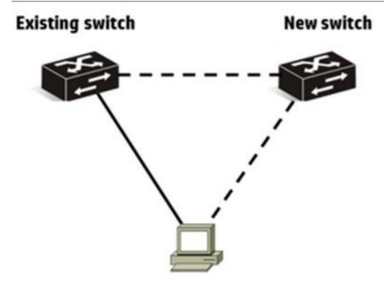
A network administrator has a server currently connected to an access layer switch. The network administrator needs link redundancy for the server and wants to add a second access layer switch and connect it to the server. Which solution should the network administrator implement to accomplish this goal?
