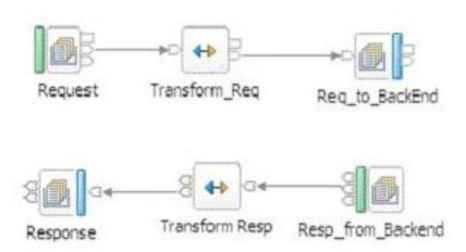
2) Synchronous, completing the round trip in the same flow pulling the response message with an MQGet node
