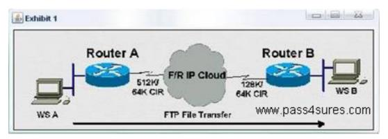
Router A has a 512K-access port into the frame relay cloud. Router B has 128K-access port into the frame relay cloud. The two routers are connected with symmetrical PVCs that are configured for 64K committed information rate (CIR). What Frame Relay Traffic Shaping map-class subcommand should be entered on Router A to prevent workstation A from overrunning the access port on Router B?
