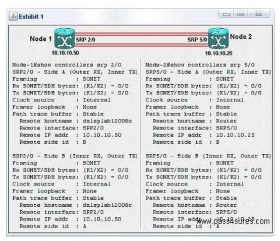
A customer has improperly installed a 2-node OC-12 SRP ring using dark fiber. Based on the printout from each node shown in the exhibit, what is the problem?
