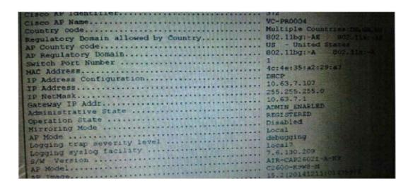
Refer to the exhibit which syslog logging facility and severity level is enabled on this AP?
