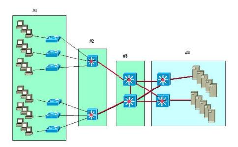
A standard, Layer 2 campus network design is pictured. Which numbered box represents the distribution layer?
