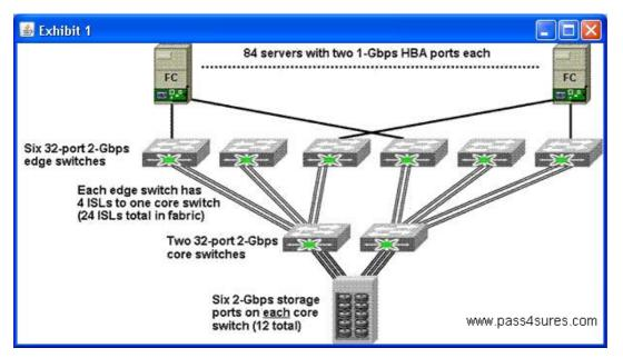
You are designing a new SAN. The existing SAN uses eight 32-port 2-Gbps Fibre Channel switches. Two of the switches are deployed as core switches, and the remaining six switches are deployed as edge switches. Each edge switch has two ISLs to each of the two core switches. The disk array has twelve 2-Gbps Fibre Channel ports. Each of the 84 servers has a dual-port 1-Gbps Fibre Channel HBA.
