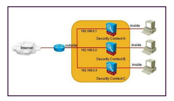
Refer to the exhibit. The Cisco ASA is dropping all the traffic that is sourced from the internet and is destined to any security context inside interface. Which configuration should be verified on the Cisco ASA to solve this problem?
