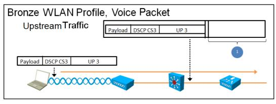
Voice signaling traffic is being sent upstream using a WLAN configured for bronze QoS. Assume that Layer 3 switches between the controller and the AP use the default and recommended CoS-to-DSCP and DSCP-to-CoS maps. What CAPWAP QoS markings are used in the header at location 1?
