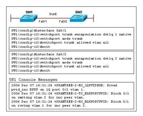
The link between switch SW1 and switch SW2 is configured as a trunk, but the trunk failed to establish connectivity between the switches. Based on the configurations and the error messages received on the console of SW1, what is the cause of the problem?
