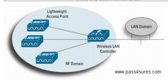
As more vendors migrate to a hierarchical design, and as larger networks are built using lightweight access points, there is a need for a standardized protocol that governs how lightweight access points communicate with WLAN systems. This is the role of the Internet Engineering Task Force's (IETF's) latest draft specification, Lightweight Access Point Protocol (LWAPP). With LWAPP, large multivendor wireless networks can be deployed with maximum capabilities and increased flexibility.
