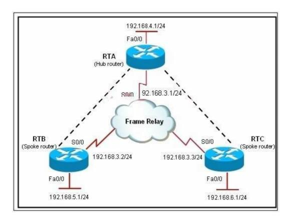
Router RTA is the hub router for routers RTB and RTC. The Frame Relay network is
