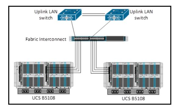
You have a virtual machine configured on each Cisco UCS B200 Series blade server installed on different Cisco UCS 5108 chassis. The virtual machines are on the same VLAN. The fabric interconnect is in end-host mode. Which statement describes how communication occurs between the virtual machines?
