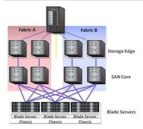
A VDC design requires 300 blade server chassis, each with two embedded Fibre Channel switches, which are connected to two separate SAN fabrics. All of the blade chassis FC switches are configured in NPV mode, and the SAN core switches are configured in NPIV mode.
