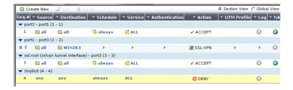
Given that the user authenticates against the SSL VPN policy shown in the image below, which statement below identifies the route that is added to the client's routing table.
