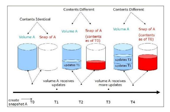
Which HP Enterprise Virtual Array snapshot concept is shown in the exhibit?
