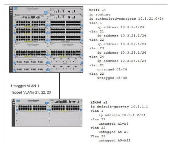
In the configuration shown in the exhibit, which users can access the web management interface of the E5406 zl?
