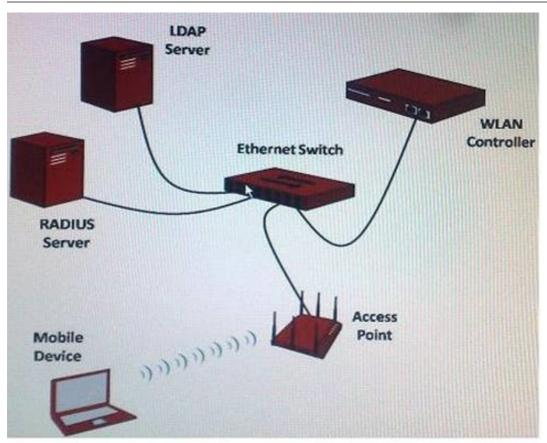
Given: The network in this diagram implements an 802.1X/EAP-based wireless security solution. What device functions as EAP authenticator?
